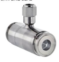
In-line seals are integrated directly into the process line. They are less temperature-sensitive than diaphragm seals and are particularly suitable for applications, which are absolutely free of dead space, with circulating, high-viscous media and with media tending to velocity and with frequent changes of the medium.
