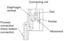
Pressure Gauge in line with Safety Requirements According to EN 837-1, S3 (formerly DIN 16 006 Part 1 and Part 2)
